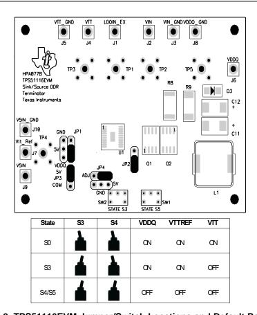
Figure 2. TPS51116EVM Jumper/Switch Locations and Default Positions
