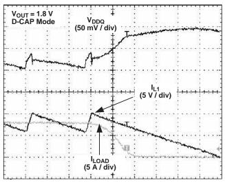
Figure 5. TPS51116EVM 0-A to 8-A Load Transient Response
