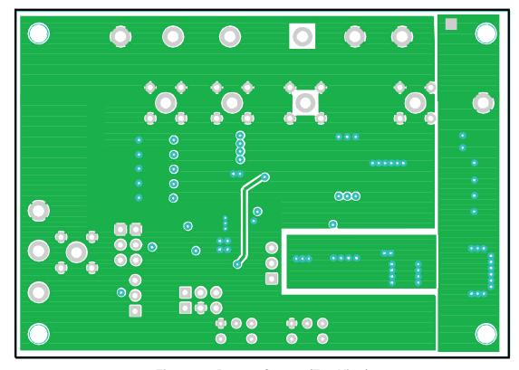
Figure 11. Bottom Copper (Top View)
