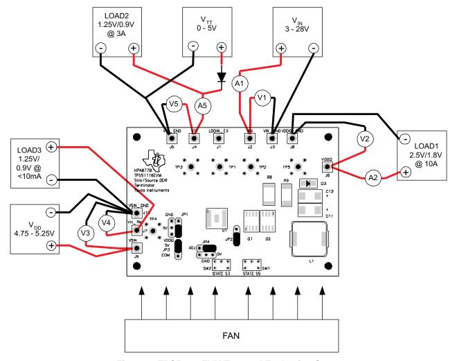
Figure 3. TPS51116EVM Test and Evaluation Setup
