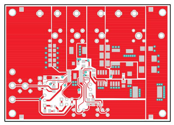
Figure 8. Top Copper Layer (Top View)
