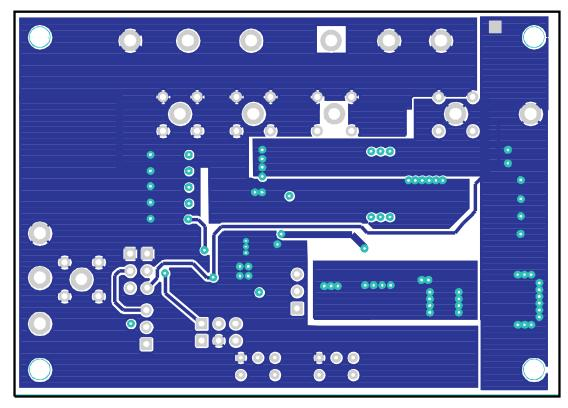
Figure 10. Internal Layer 2 (Top View)
