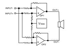
Figure 1: APA2030 Internal Configuration (each channel)
