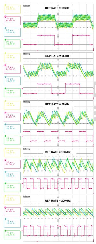
FIGURE 11. CURRENT BALANCING DURING DYNAMIC OPERATION. CH1: IL1, CH2: IL0AD, CH3: IL2, CH4: IL3
