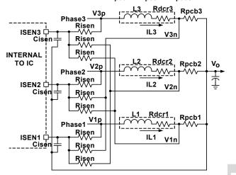
FIGURE 10. DIFFERENTIAL-SENSING CURRENT BALANCING CIRCUIT
