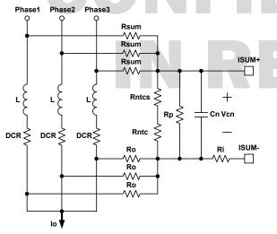
FIGURE 15. DCR CURRENT-SENSING NETWORK
