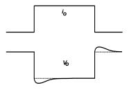
FIGURE 17. LOAD TRANSIENT RESPONSE WHEN  $\mathbf{C}_{\mathbf{n}}$  IS TOO SMALL
