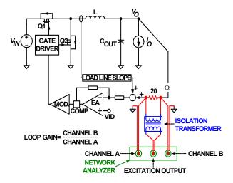
FIGURE 24. LOOP GAIN T2(s) MEASUREMENT SET-UP
