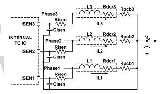
FIGURE 9. CURRENT BALANCING CIRCUIT
