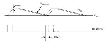
Figure 5—Jitter in Skip Mode
