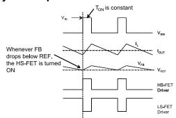
Figure 2—Heavy Load Operation
