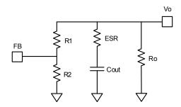
Figure 8—Simplified Circuit in skip Mode
