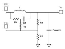
Figure11—Simplified Circuit of Ceramic Capacitor
