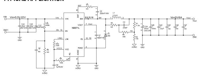
Figure 14 — Typical Application Circuit For NB671L  $V_{IN}$ =5.5-22V,  $V_{OUT}$ =5V,  $I_{OUT}$ =6A
