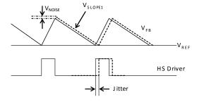
Figure 4—Jitter in PWM Mode
